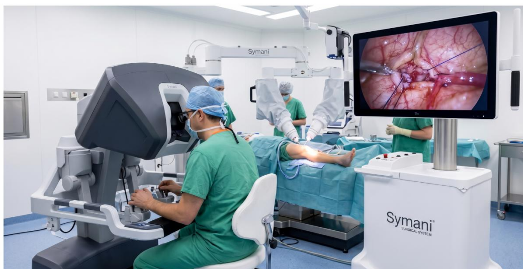
Figure 4. Robotic-Assisted Supermicrosurgery. The Symani Surgical System, a dedicated supermicrosurgical robotic platform featuring motion-scaling and tremor reduction, utilized to perform high-precision lymphovenous anastomoses (13).
